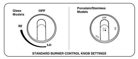
All the controls are push in to turn and have an infinite number of heat settings, with no fixed positions. Select the appropriate control knob and turn it counterclockwise to the **HI** position (detent) until the burner lights. Adjust the flame size. Turn off by turning the control clockwise to **OFF**.
